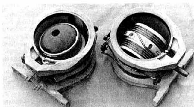
HF variometers as used in the German FuG10 aircraft transmitter-receiver initially designed and built by Lorenz from 1937. Normally these units had powder iron cores as shown in the unit on the left. When the core was removed for post-war amateur equipment as in the unit on the right it reduced the maximum inductance from 38 to 17 \mu H. Mechanical construction made such units suitable for high-stability variable frequency oscillators. (Photograph courtesy DL6KG)
