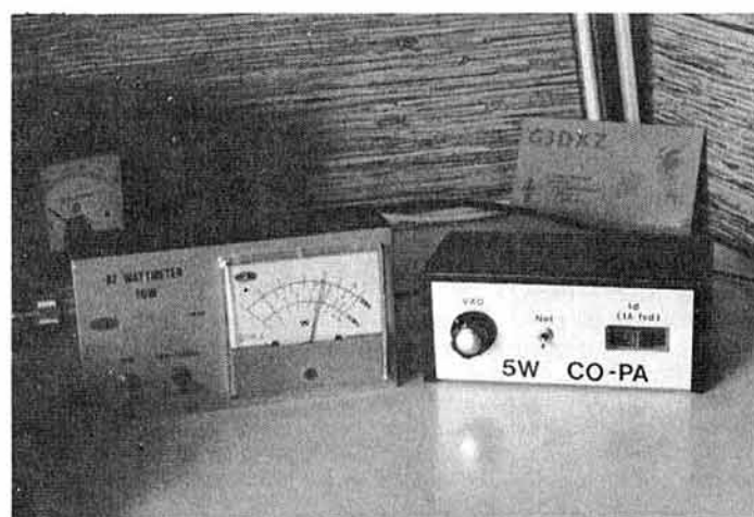
Transmitter, coupled to a power meter, under test
